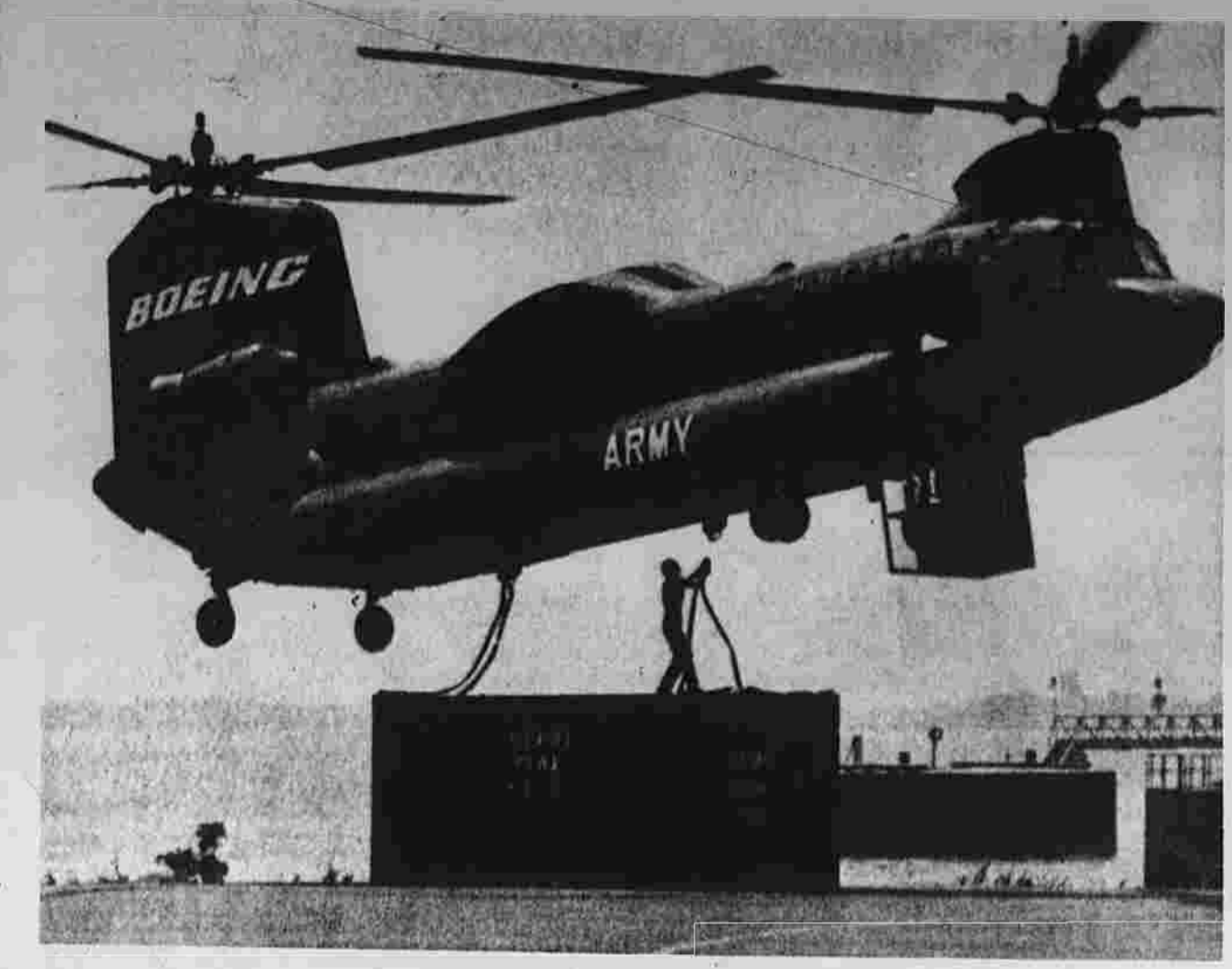
Checking Out Chopper A ground crewman makes the final hook up as a Boeing heavy-lift helicopter tests its ability to lift cargo while in flight. The control of the helicopter during the lifting operation is shifted from the pilot's cabin to control cabin under the craft. The test was made at the Boeing plant in Philadelphia. (UPI photo)
